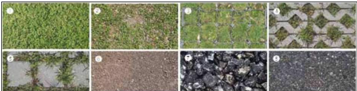
Figure 82: Overview of most common ground surfaces, from most to least permeable (European Union, 2013)
